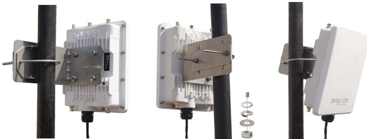
Figure 4-3 Pole Mounting (MP-1015 & MP-1025)
